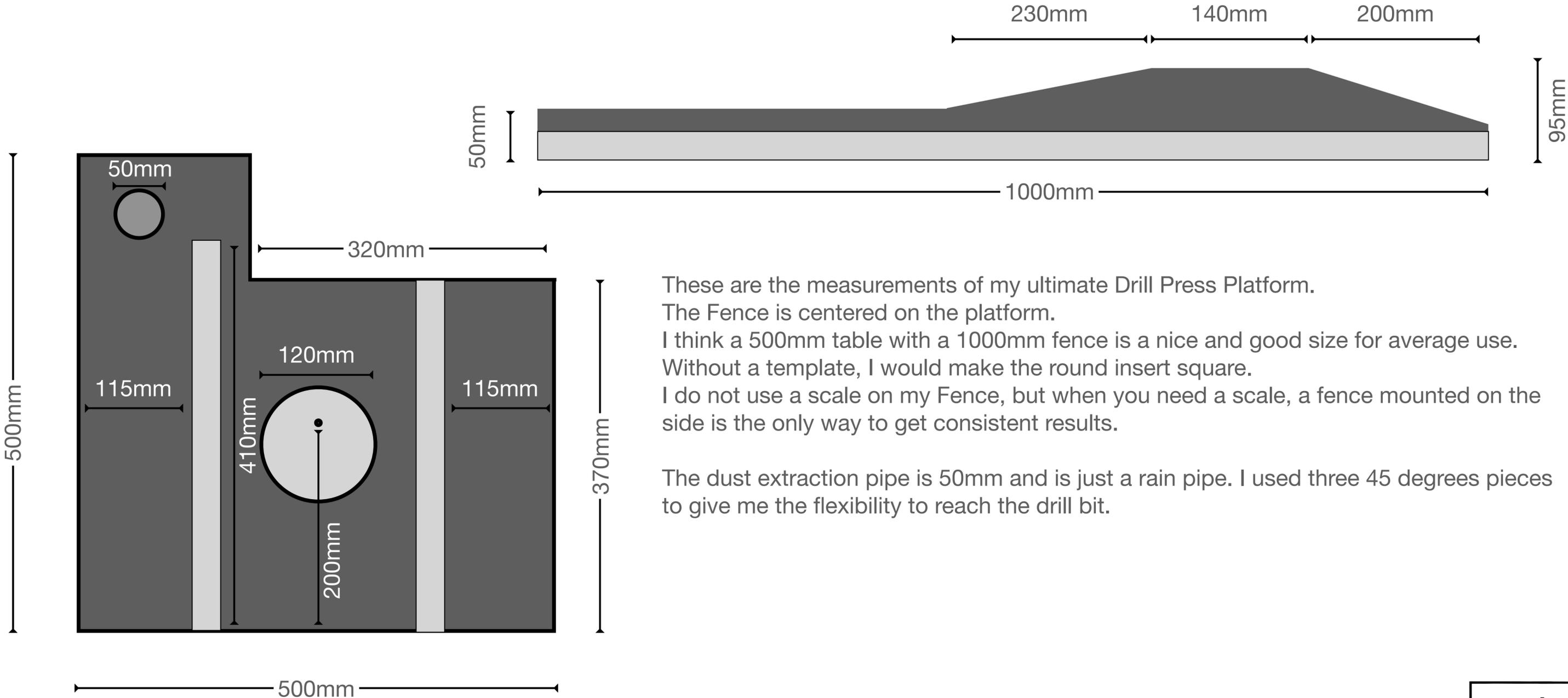
These are the measurements of my ultimate Drill Press Platform. The Fence is centered on the platform. I think a 500mm table with a 1000mm fence is a nice and good size for average use. Without a template, I would make the round insert square. I do not use a scale on my Fence, but when you need a scale, a fence mounted on the side is the only way to get consistent results.
